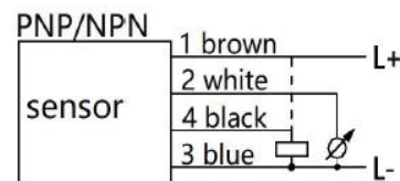
1 switching output + 1 analog output
